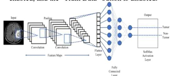
Figure 2. CNN Layers for the proposed model.
