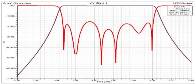
Fig.3 S parameter(dB) versus Frequency of Microwave Bandpass Filter
